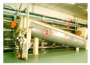
At the output of the mill, the cocoa powder is hot and needs to be cooled down to prevent fat blooming and powder lumping
